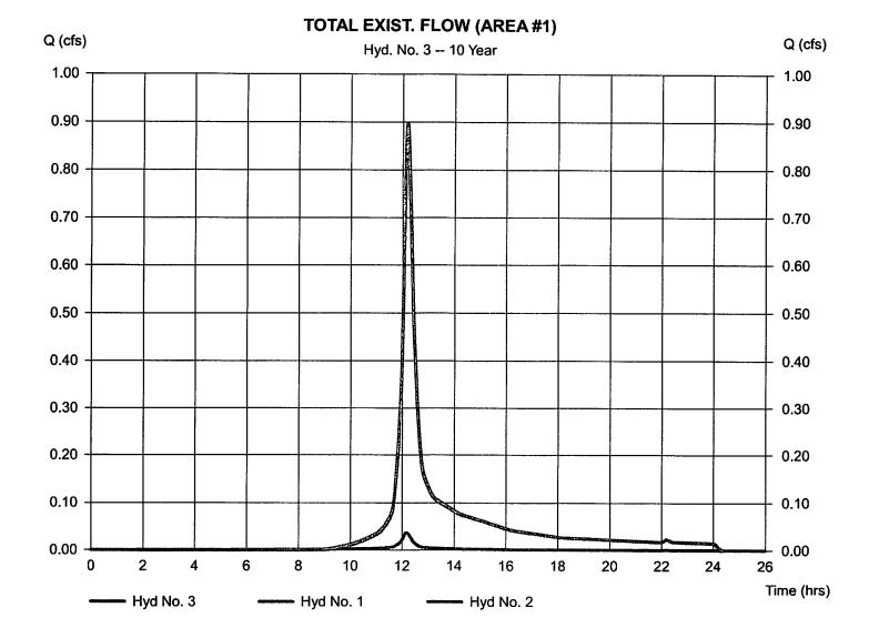
Hydraflow Hydrographs by Intelisolve v9.2
